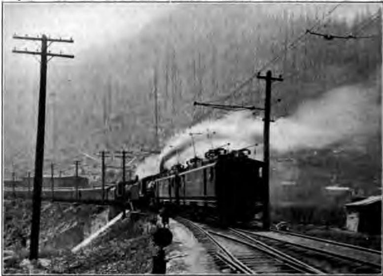
TWO TRIPLE-PHASE LOCOMOTIVES OF THE GREAT NORTHERN RAILWAY HELPING A DOUBLE-HEADER STEAM TRAIN UP THE GRADE INTO THE CASCADE TUNNEL
